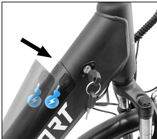
2. Connect the battery socket to the pin and push it up, Turning the key to the "lock" position.
